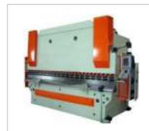
CNC BENDING Capacity upto 8 mm 12 mtr length
